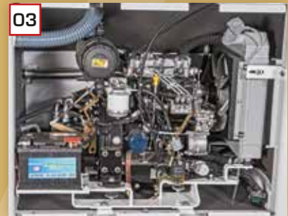
03 Powerful watercooled 3 cylinder turbulence chamber four stroke suction diesel engine by Kubota
