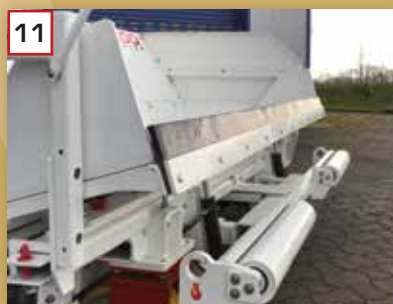
Hydraulic lift adjustment of the bunker flap
