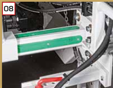
Hydraulic screed levelling
