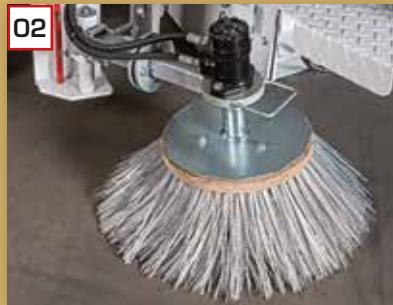
02 Disc broom for cleaning the road pavement (optional)
