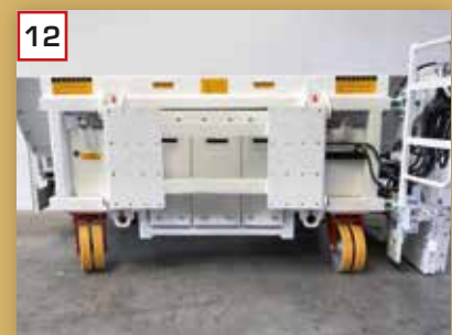
Universal adapter plate to connect the wheel loader or tractor (optional)
